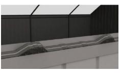
Step 2: The inside Closure fits the underside of the panel.
