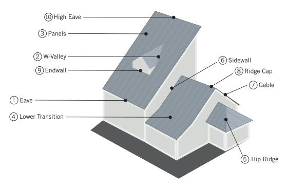
Installation over shingles is not recommended. It is best to remove shingles and install a new, synthetic underlayment to act as a vapor barrier between the substrate and the metal. If shingles will not be removed, furring strips need to be installed on the roof at 2'-0" centers. The metal panels will then be fastened to the furring strips.
